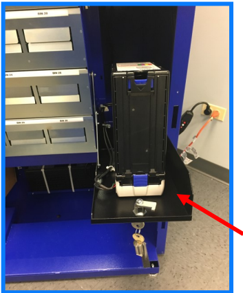
3. Guide the unit down avoiding letting it slam down.
