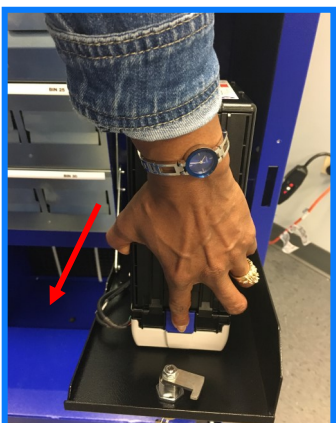
5. Holding the button, pull the Cashbox forward.
