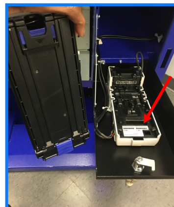
6. The unit will detach from the base.
