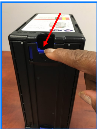
3. Push down on blue button to release Cashbox door.
