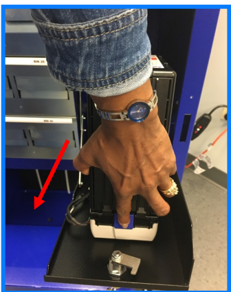
5. Holding the button, pull the Cashbox forward.
