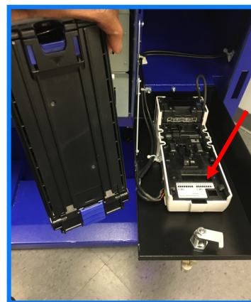
6. The unit will detach from the base.
