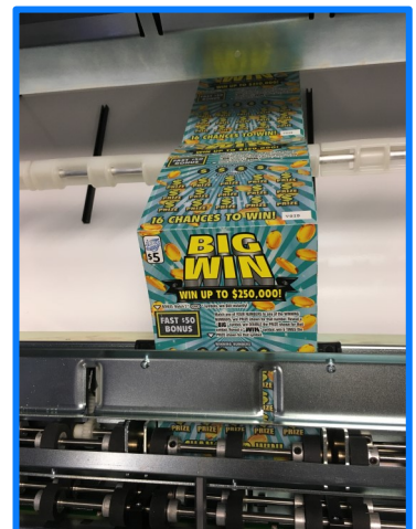
6. Tickets will be properly seated by burster.
